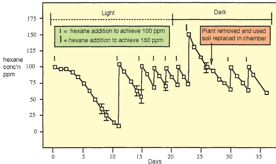
Fig.2. n-hexane levels in air of test chambers containing *Dracaena* var Janet Craig plants maintained in potting medium (soil).
